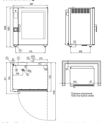
Heat Source: 500mm clearance from an external heat source is required in order to protect the oven control components and allow access to the service panel. For clearances under 500mm, it is mandatory for Stoddart heat shields to be fitted while still maintaining a minimum clearance of 300mm to provide access to the service compartment. Failure to adhere to minimum clearances may void the oven warranty or add service costs due to lack of access.
