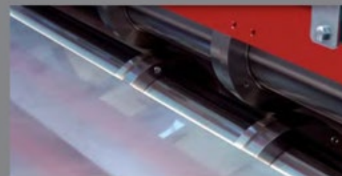
Cutter spindle with 100mm diameter
