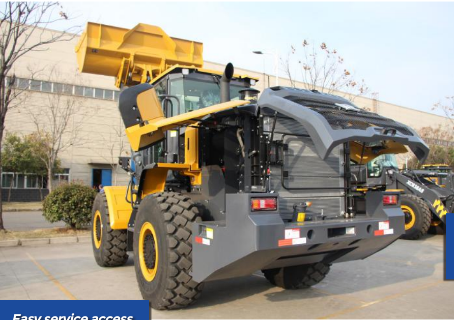
Easy service access to all componentry
