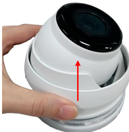
Remove the Outer Housing
