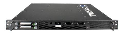
**Field tested, fail-safe and long-life performance in extreme conditions.** As processing performance continues to improve, Crystal Group is dedicated to minimize the SWaP envelope of the RS112S14. High-end computing performance in a 1U chassis with a depth of 13.4" (34.04 cm) fits most any rack space.
