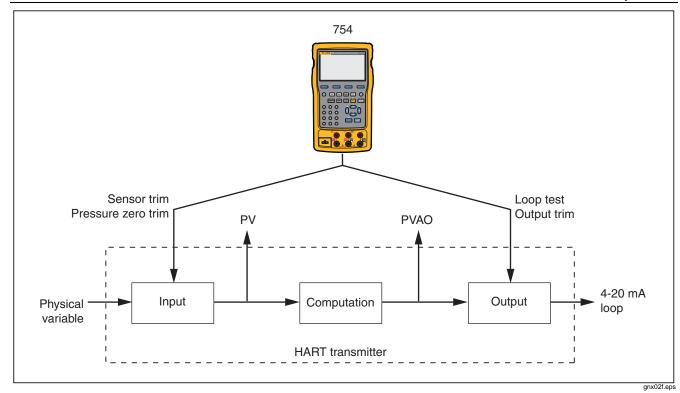
Figure 12. Block Diagram of a HART Transmitter
