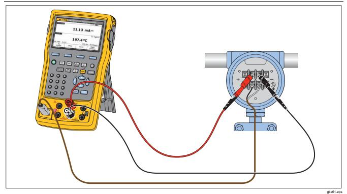
**Figure 3. HART Transmitter Connection**
