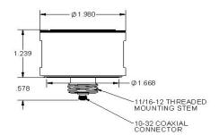
Units on the line drawing are in inches, units in brackets are in millimeters. Refer to 127-1060V for more information.
