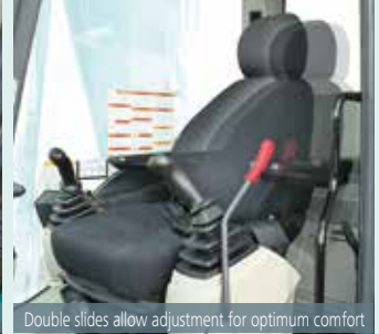
Double slides allow adjustment for optimum comfort
