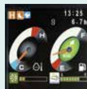
PM accumulation/ Urea accumulation display
