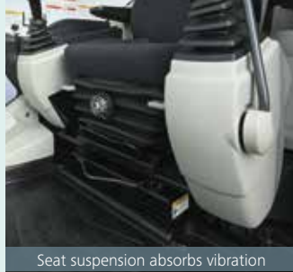
Seat suspension absorbs vibration
