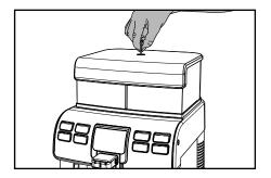
2 After unlocking the lid, lift and remove it.
