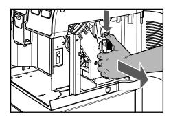
5 Wash the Brew Group with lukewarm water and carefully wash the upper filter. Before placing the Brew Group in its seat, ensure that there is no water left in the brewing chamber.
