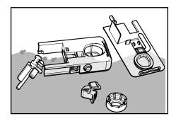
**15** After washing, reassemble the parts following the same procedure used for disassembly, but in reverse order.
