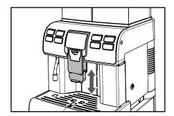
Manually move the dispensing spout up or down to adjust its height.
