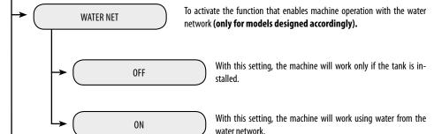
Note: Use this function with utmost care, as a wrong setting may cause malfunctions. The "ON" option must only be activated if the "WATER NET" kit is installed and connected properly. Using it under any other conditions will result in a machine failure.
