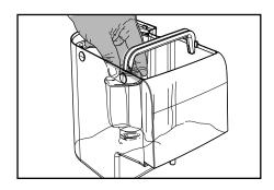
13 Fill the tank with fresh drinking water and reinsert it into the machine.
