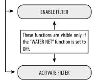
To activate/deactivate the warning indicating that the water filter should be replaced. By activating this function, the machine notifies the user when the water filter needs to be replaced.
