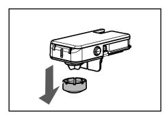
Turn and lift the Cappuccinatore cover and remove it from the Cappuccinatore body.
