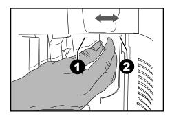
The reference marks indicate the grind setting. You can set different degrees of grind with the following references:
