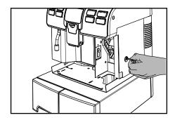
4 Remove the Brew Group: Pull it by the handle and press the «PRESS» button. The Brew Group must be washed only with lukewarm water, with no detergent.
