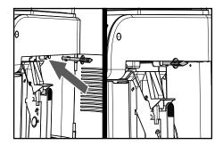
Warning! Disabling the safety microswitch entails a danger for the operator to come into contact with the moving parts of the appliance. Enable the safety device again right after completing the adjustment.
