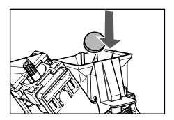
**12** After placing the tablet in the brew group press the "**"** button (18) to confirm.
