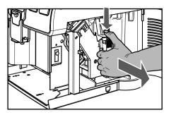
4 Lift the rear side of the inner drawer and unlock the drawer.
