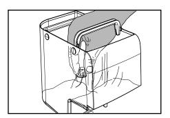
12 Put the filter into the empty tank. Press it until its limit stop.
