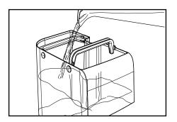
9 Place the tank back in the machine. Press the "<u>P"</u> button (18).
