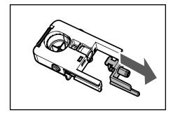
13 Remove the suction tube joint from the Cappuccinatore.
