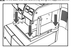
Remember that the components must be correctly aligned: Check them.
