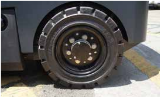
Equipped with EXMILE 4.00-8 super-elastic solid tyres which ensure good performance and extended life.
