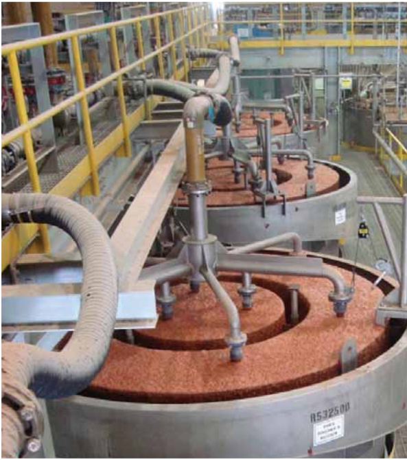
▲ Column flotation cells recover fines material in processing operations.
