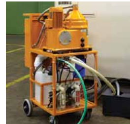
Portable Centrifuge Removes free and emulsified tramp oils through a high speed centrifuge
