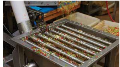
Grate Magnet used in food preparation at Better Baked Foods in Pennsylvania. Grate Magnets provide powerful, permanent protection against fine and tramp iron contamination... from simple tubes to fully automated tramp metal removable designs.
