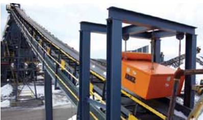
Suspended Electromagnets safely and automatically remove tramp iron from heavy product flows such as wood, coal or aggregate being conveyed on belts, vibratory feeders or in chutes.
