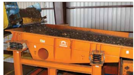
Mechanical Feeder presents an even flow of material to an automated sorter at a scrap yard.
