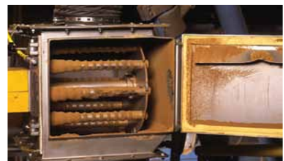
Magnetic Rota-Grate® removes metal contaminants from dry process flows. This in-housing design is ideal for dusty installations where an enclosed system is necessary. The slowly rotating tube circuit catches unwanted tramp iron and prevents bridging of powdery material like flour.
