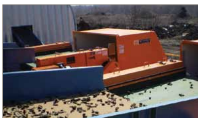
Powerful Eddy Current Separators utilize Rare Earth magnets arranged into high speed, composite-shelled rotor to deliver exceptional nonferrous metal separation from PET flake and bottles.
