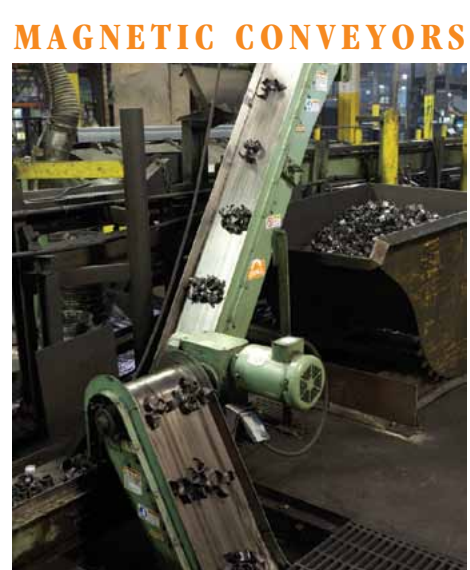
Magnetic Conveyor transports steel "knock-out" scrap from forming press in Pennsylvania.
