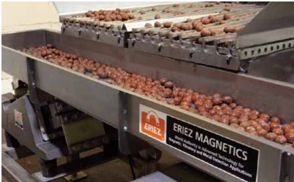
▲ A New York-based manufacturer of chocolates uses vibratory feeders and conveyors to process candies.
