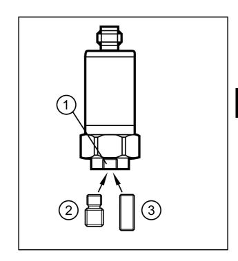
The measuring direction should be in the direction of the main vibration. The main vibration is usually in radial direction to the shaft.
