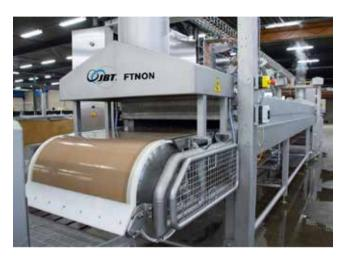
Steam tunnels with Teflon coated Kevlar belt:
