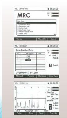
All methods are included as built-in standard; this eliminates the need of software. Online software update via Internet. The local control software includes functions such as: Photometry, Quantitative, Wavelength Scan, Kinetics, DNA/Protein, Multi-wavelength and System Utilities.
