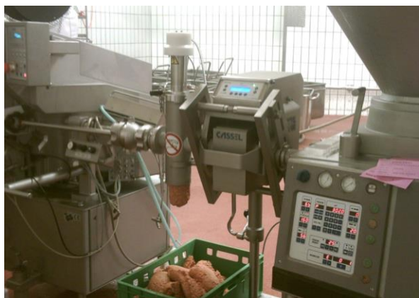
METAL SHARK® IN Meat fitted into a production line.
