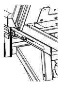
Pull the black bolt to adjust the stroke, then lock again
