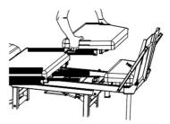
• Step 2: Turn the black handle into the unlock position & the back section can then slide on the track.
