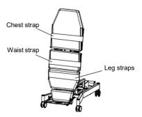
Tighten the belts by fastening the straps. The position of the straps can be moved up and down along the square tube.
