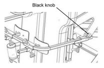
• Step 2: Put the knee pad into the frame adjusting to the tube 1 is used to adjust the gap between the knee pad to knee.
