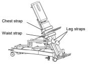
Tighten the belts by fastening the straps. The position of the straps can be moved up and down along the square tube.
