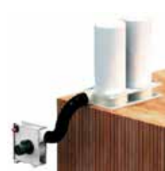
301-007 Chip Extraction System for Chip Containers Complete extraction system that includes filter, cyclone and chip collection bags. For use with a chip container. Delivery hose between cyclone and fan allows the fan to be located away from the cyclone system. Collection bag size is 2 x 250 litres. (for MP260 and MP160)
