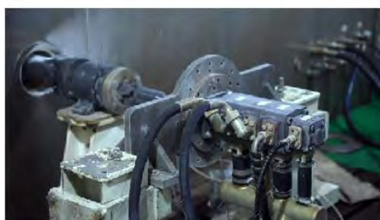
Hydraulic oil pump Low-temperature performance test under -40 /
