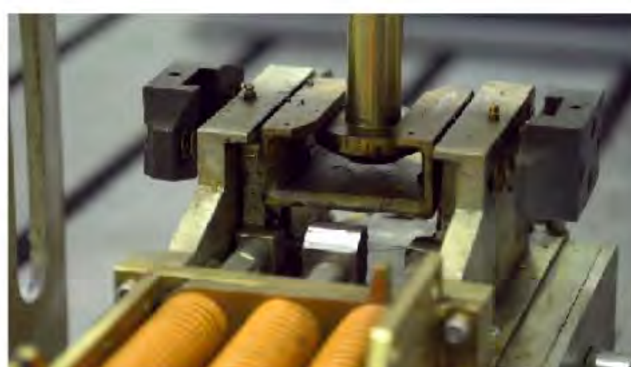
Telescoping mechanism Smoothness test
