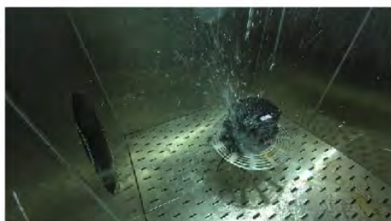
Length measurement sensor 48-hour rain-proof test
