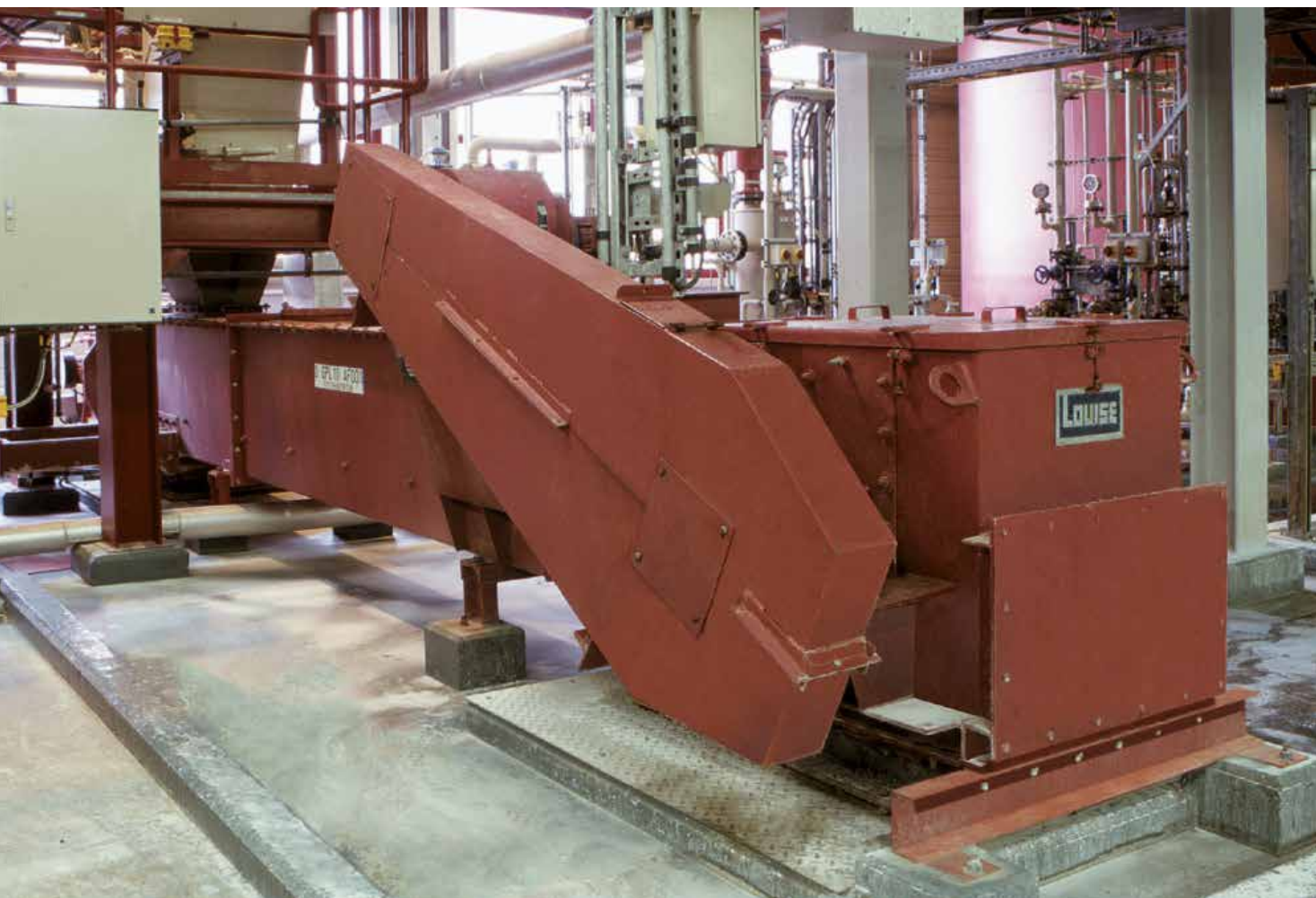
A double-strand Chain Conveyor loads FGD Gypsum from the flue-gas desulphurisation into the storage silo
