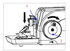
As the drawing shows , turn the handwheel (2) to drive the specimen clamp(1) moving in the vertical direction.
