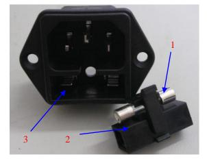
• put the fuse (1) in the installation part (2) and then insert the installation part into the socket(3).
