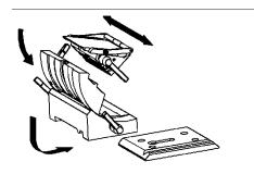
Take down all the parts of the knife holder as it is showed in the picture and then cleaning all the parts separately especially the following easily polluted parts: the slider, lever, blade clamp and the joint of the parts. And remember to clean the blade clamp every time before install the blade to ensure getting a good sectioning.
