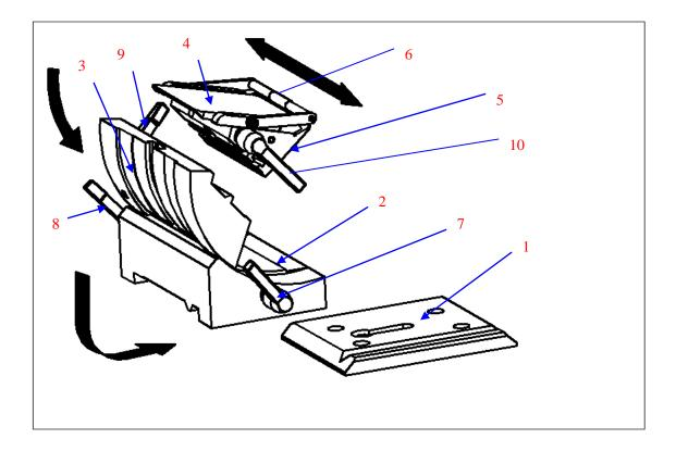
As the drawing shows, the knife holder be composed of the following parts: Z axis slider (1), Y axis slider (2), X axis slider (3), clamp2 (4), clamp1 (5), knife guard (6), lever 2 (7), lever 2 (8), lever 2 (9), lever 1 (10).
