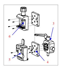
As drawing shows, the specimen clamping system is made up of adjustor(3), connect board (4) and clamp(5, 6).
