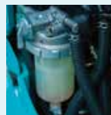
Pre fuel filter with built-in water separator
