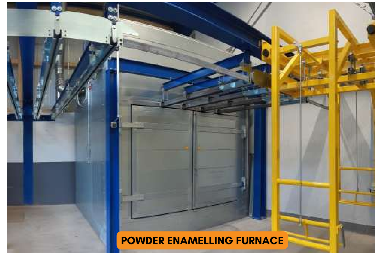
Powder enamelling furnace with a circulating air heating of up to 230 °C
