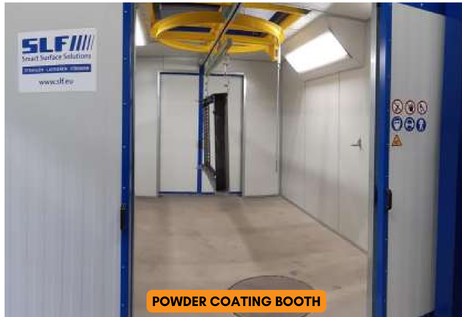
Powder coating booth with laterally installed cartridge filter unit and 2 sliding doors designed as entry and exit door
