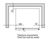
Heat Source: 500mm clearance from an external heat source is required in order to protect the oven control components and allow access to the service panel. For clearances under 500mm, it is mandatory for Stoddart heat shields to be fitted while still maintaining a minimum clearance of 300mm to provide access to the service compartment. Failure to adhere to minimum clearances may void the oven warranty or add service costs due to lack of access.
