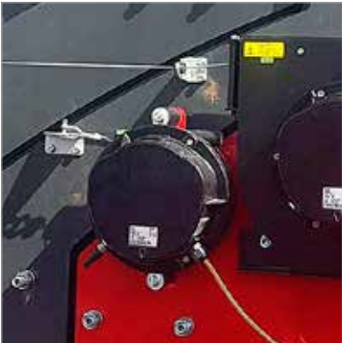
Potentiometer for angle and length of boom detection with redundant safety.
