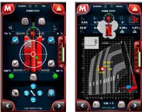
Dynamic representation of all the collected data on the touch screen for the operator.
