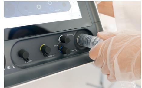
Canopy tests require a simple set-up by connecting the canopy hose to the blower
