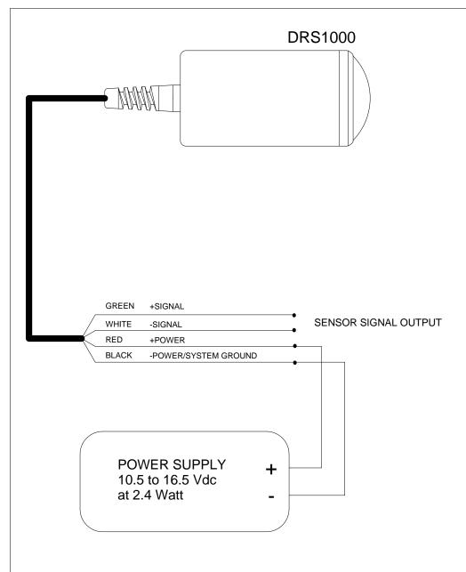
The signal output from the DRS1000 speed sensor is a 0 to 5 volt differential line driver that is compatible with RS485 specifications. The sensor output may be interfaced to the monitoring electronics in a number of ways:
