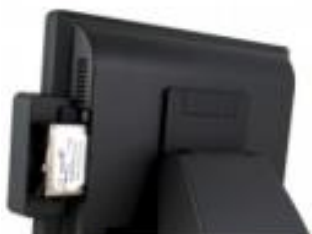
Slide in/out HDD Replacement
