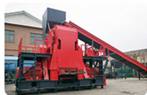
Material: Cast Aluminum Solutions: Shredding+Separating Area: Tunisia
