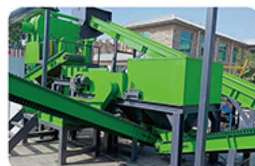
Material: Steel Scrap Solution: Shredding+Separating Area: South Africa
