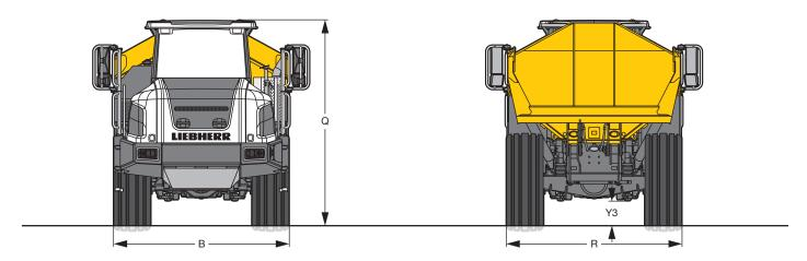
Transport Dimensions Incl. option for dump body flap and including special tires
