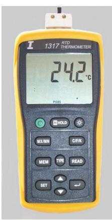
Data Logger model includes software & PC Interface (T1317R- 4200 Records)
