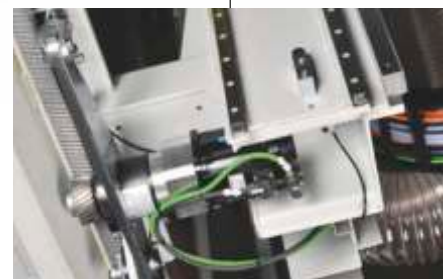
Lower gantry motor
