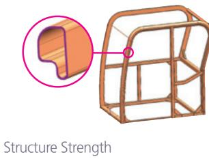
The R80CR-9 cabin structure has been fitted with stronger but slimmer tubing for added safety and improved visibility. Low-stress, high strength steel is integrally welded to form a stronger, more durable upper and lower frame. Structural integrity was tested by way of FEM (Finite Elements Method) analysis and long-term durability tests.
