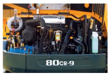
The R80CR-9 is equipped with a durable plastic air cleaner designed
