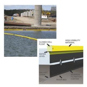
The Absorb Floating Silt Curtain contains silt runoff in streams by acting as a floating barrier. The floats are closed cell polyurethane and are encased in a high visibility yellow material. It is made from a non woven geo-textile with a mean aperture of 120 microns. Standard Floating Silt Curtains come in 2m deep and equipped with a ballast pocket at the bottom and heavy duty chain as ballast.
