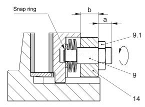
Fig. 25 Cup spring supporting bolt (9) with counter nut (9.1)
