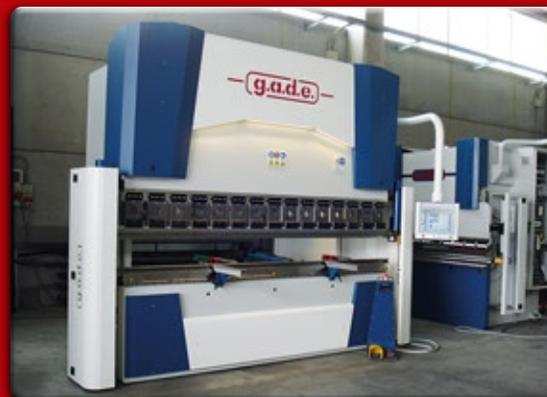
The PE and PE-C electric press brake range was developed thanks to a cooperation between g.a.d.e. and MechLav Laboratory specialized in the advanced mechanics, an engineering department related with the University of Ferrara. In concept this kind of press brakes applies the principle of an electrical hoist with pulleys connected in series which move the tool holder (top beam) through high resistance drive belts.
