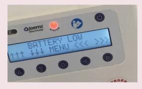
LOW BATTERY - For Inline charge systems the lift unit will charge anytime the hoist is not in use. When the batteries charge level reaches a low condition, the charge / status indicator will flash red and, in ambient light conditions, this will be accompanied by an audible beep each time an operating control is depressed. In low light conditions, only the charge / status indicator will flash red.
