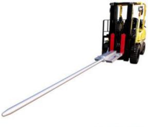
Slip-on and carriage mounted Carpet poles suitable for moving fabric, cable and coil products by forklift. It can also be used for carpet handling, but usage is generally restricted to larger forklifts due to the extended load centre created by the length of the tines.
