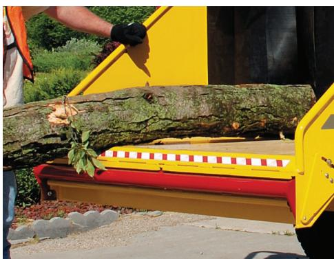
**BOTTOM FEED STOP BAR.** Strategically located to make it possible for an operator's leg to strike the bar and shut off the feed mechanism, either intentionally or automatically in an emergency situation.
