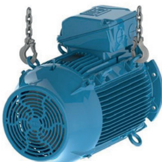
Figure 4.20 - Final result: motor placed in horizontal position
