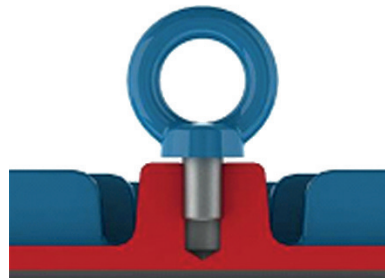
Figure 4.2 - Incorrect tightening of the eyeboll
