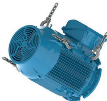
Figure 4.19 - Motor is being rotated to horizontal position
