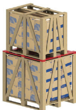
Figure 5.5 - Use of additional battens for stacking
