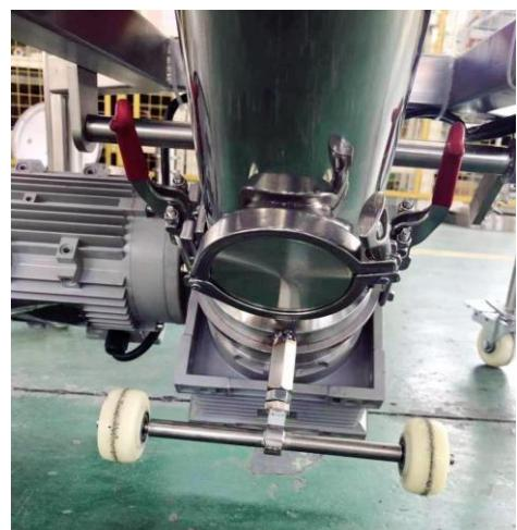
3. The residue discharge port with a door at the bottom of the tube, makes it easy to clean the residue without dismantle it.
