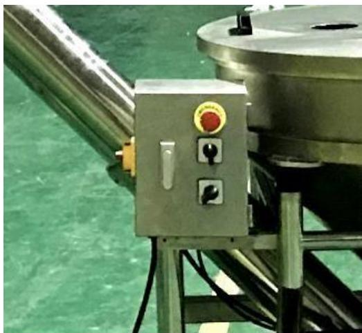
7. SUS304 electric cabinet. Two black switches on the feeder. One to turn the auger, one to vibrate the hopper.
