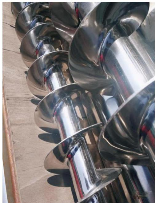
2. The conveying pipe is stainless steel 304, full weld and full mirror polishing. It is easy to clean, and no blind area to hide material.
