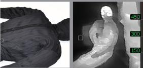
We have designed a special suit which goes over the top of your existing manikin to give instant thermal imaging capabilities.
