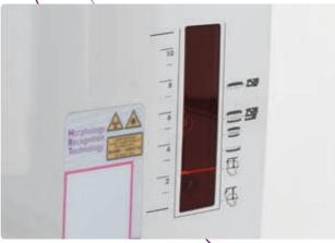
The icons provide a valuable visual reference, ensuring correct positioning of the horizontal laser according to the scan type and, therefore, maximum diagnostic accuracy for 2D, 3D and CEPH images.
