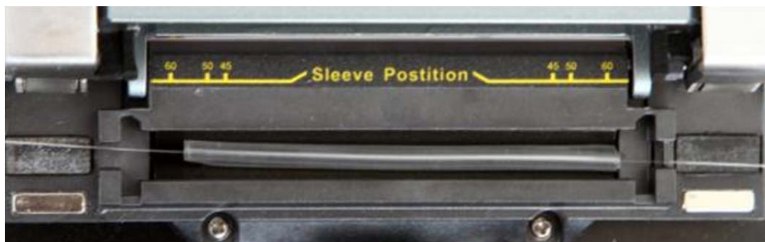
Heater and detection unit
