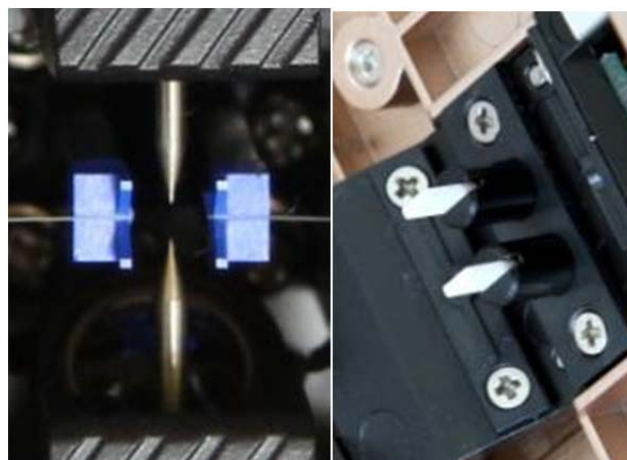
High-precision ceramic V-groove and presser foot
