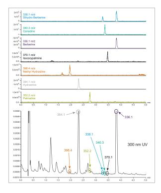
By adding mass detection with the ACQUITY QDa Detector to an existing Alliance HPLC System with UV detection, the peaks of interest in this Golden Seal sample can be easily identified by their m/z values. The mass analysis window in Empower 3 Software allows you to easily review UV and MS data in a single view.
