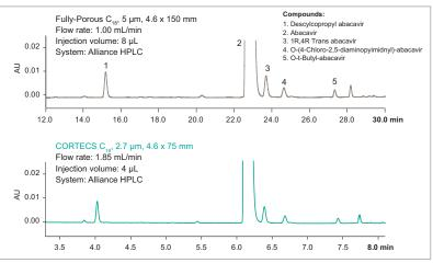
The method for Abacavir is transferred from a fully porous 5  $\mu$ m C<sub>18</sub> to a CORTECS C<sub>18</sub> 2.7  $\mu$ m with a 4x reduction in run time and equivalent resolution, both on an Alliance HPLC System.
