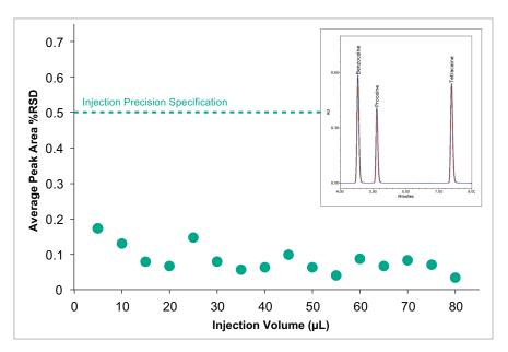
Average peak area %RSD for six replicate injections is plotted as a function of injection volume. Across the entire volume range, the injection precision is below 0.2% and well below instrument specification. Inset shows and overlay of six replicate injections at 50  $\mu$ L.
