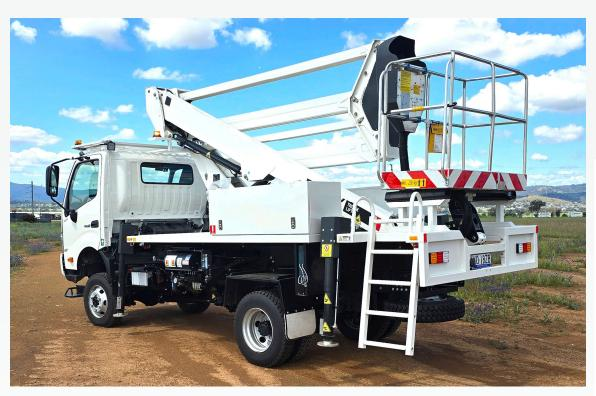
The E209PX is a super compact 20 m truck mounted lift. This versatile package is a favourite with tree trimming & trades industries. The compact boom is made up of a double articulating boom giving straight "Plumb line" movement making it great for working up a vertical face such as the side of a building. The top section is telescopic providing point and shoot functionality providing 9m outreach. With almost zero tail swing, it is well adapted to work roadside and in confined spaces.
