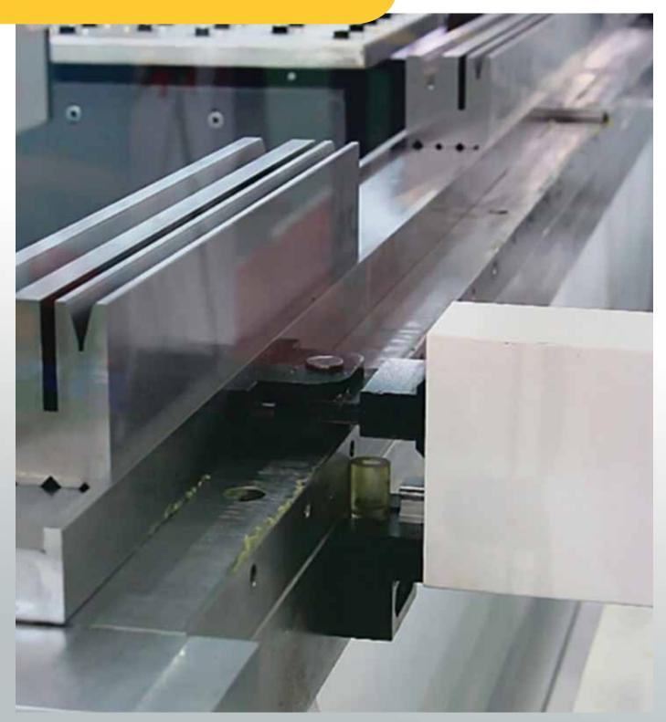
P1P2 Servo controlled table, to easy complete small bends, Using different V-openings in a die. Accurate positioning and reduced tool changes
