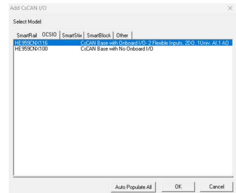
8. Now modules can be added via the "Add Module" button. As I/O modules are added the Input Map, Output Map, and Current Draw are updated, showing the accumulated I/O Module Information. More details regarding each module can be viewed via the "More Info" button.
