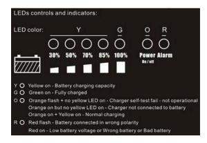
Charging shown by orange Power LED and orange Charge LEDs. The batteries are charged once the indicated LED shows 100%
