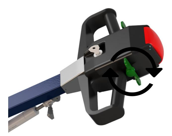
Drive the unit by moving the throttle in the desired direction. In Order to stop the unit, let go of the throttle.
