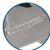
Fill welding for infection control
