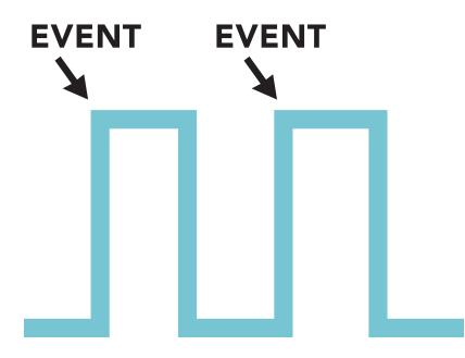
The amount of liquid moving through the flow meter is quantified by the frequency that the flow meter outputs. This is known as the flow meters K-factor.
